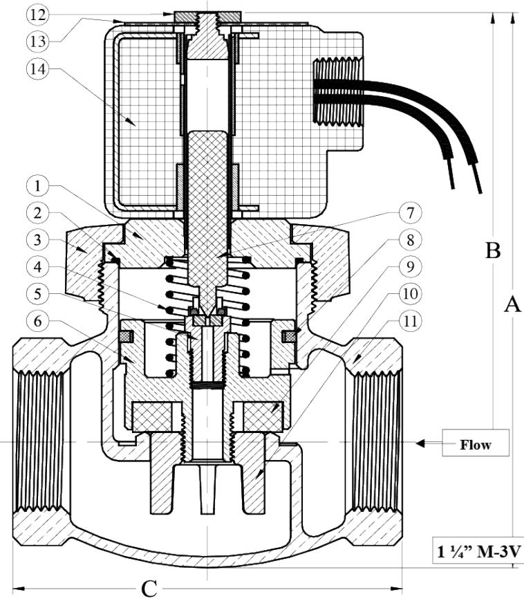
**Operation:** Piston pilot operated, minimum pressure drop of 5psi or 10psi ( $\Delta P$ ), depending on pressure rating, is required across valve for operation.
